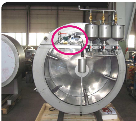
Water mixing and dosing system
