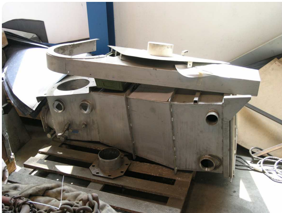
Mixing box with pipe connections and cover of chain drive.
