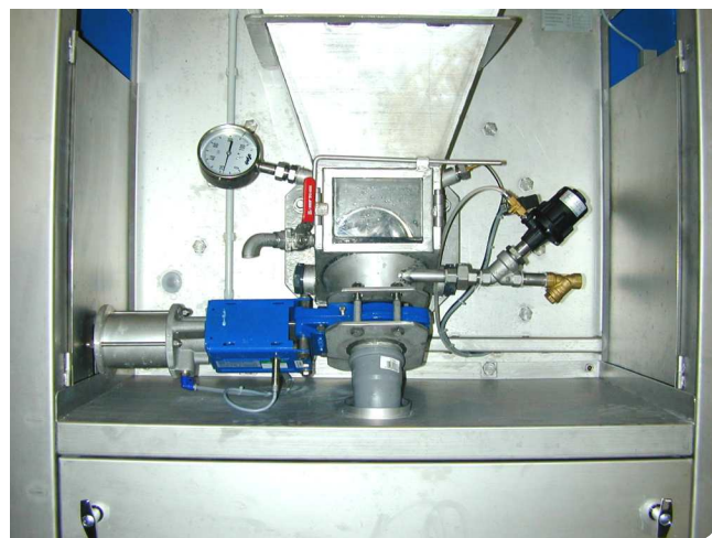
Mixing box with draining and steam connection
