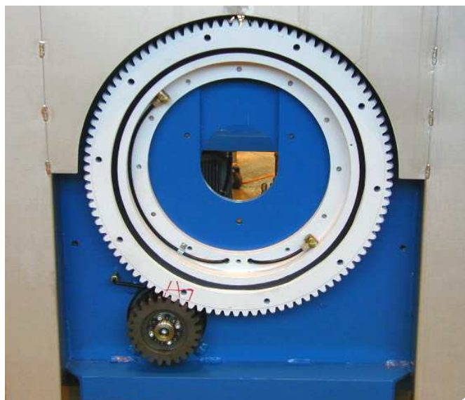
Gear wheel drive on a robust long life steel girder
