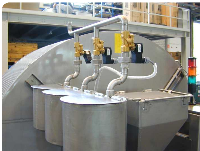
Chemical tanks with automatic dosing
